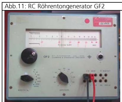
Abb.11: RC Röhrentongenerator GF2
